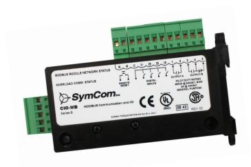
The CIO-MB/CIO-120-MB communications module is a convenient and cost-effective Modbus/RTU interface capable of providing discrete control and monitoring of a 777 Plus Series overload relay/power monitor over a Modbus network. This device can also be used as stand-alone device in MCC (motor control center) or enclosed starter applications. The CIO-MB and CIO-120-MB are designed to provide the following benefits in both new and existing installations:
